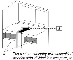
wooden strip, divided into two parts, to allow free passage of air
